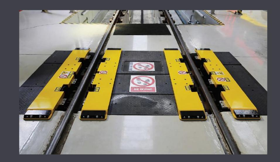
The laser measuring system for wheelsets is designed for monitoring of wheel profile wear. The degree of wheel profile wear is determined on the base of a virtual picture of wheel surface created from the measured data.\*
