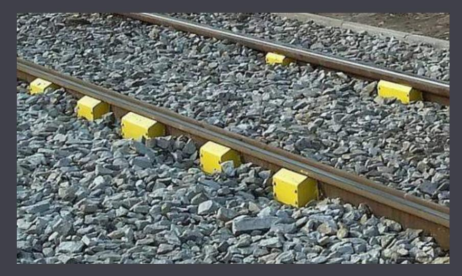
The laser measurement system for wheelsets is designed for monitoring of wheel profile wear. The degree of wheel profile wear is determined on the base of a virtual picture of wheel surface created from the measured data.\*
